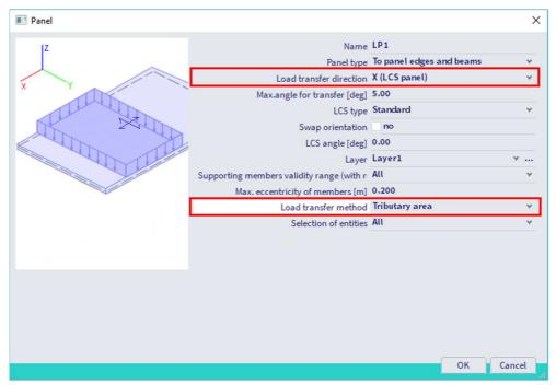
Use the snapping points in the roof to create a load panel for each pitch of the roof.
