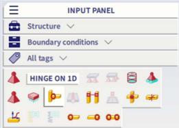
The hinges are put to both ends of the diagonals; therefore choose **Both** for the **Position** when dialogue **Hinge on beam** pops-up.
